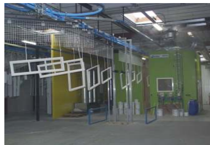
Power free conveyor
